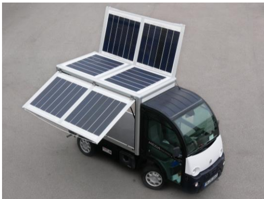
Figure 18: Fraunhofer ISEs Mega electronics e-worker with PV-box body
